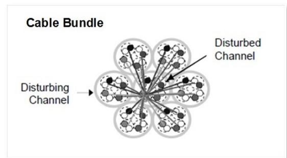
Figure 6. TIA 568-C.2 Alien Crosstalk Test Setup
